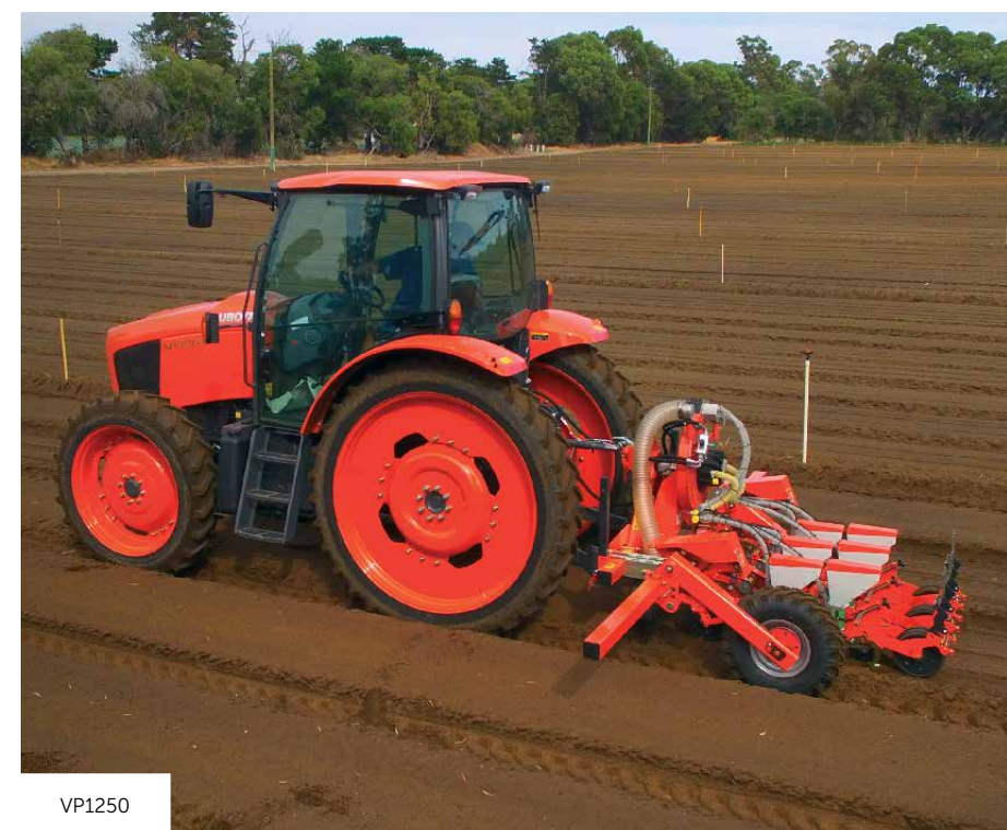
HD-II VACUUM SOWING ROW FOR PRECISE SEED SINGULATION
