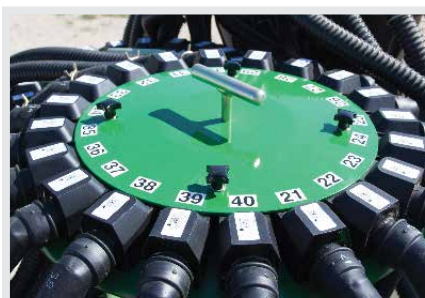
INTEGRATED BLOCKAGE SENSORS AS STANDARD
