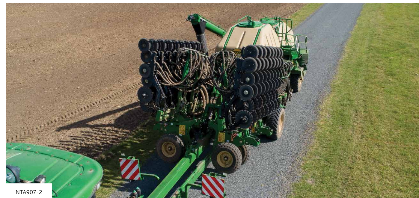
07 SERIES NO-TILL OPENER WITH 5/8" TURBO COULTER
